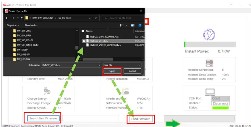
After confirming the File and clicking on the LOAD FIRMWARE button, the update procedure will begin and the HV BOX will be updated to the latest version.
