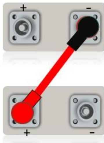
The low voltage screw terminal only supports parallel connection with maximum voltage 60V
