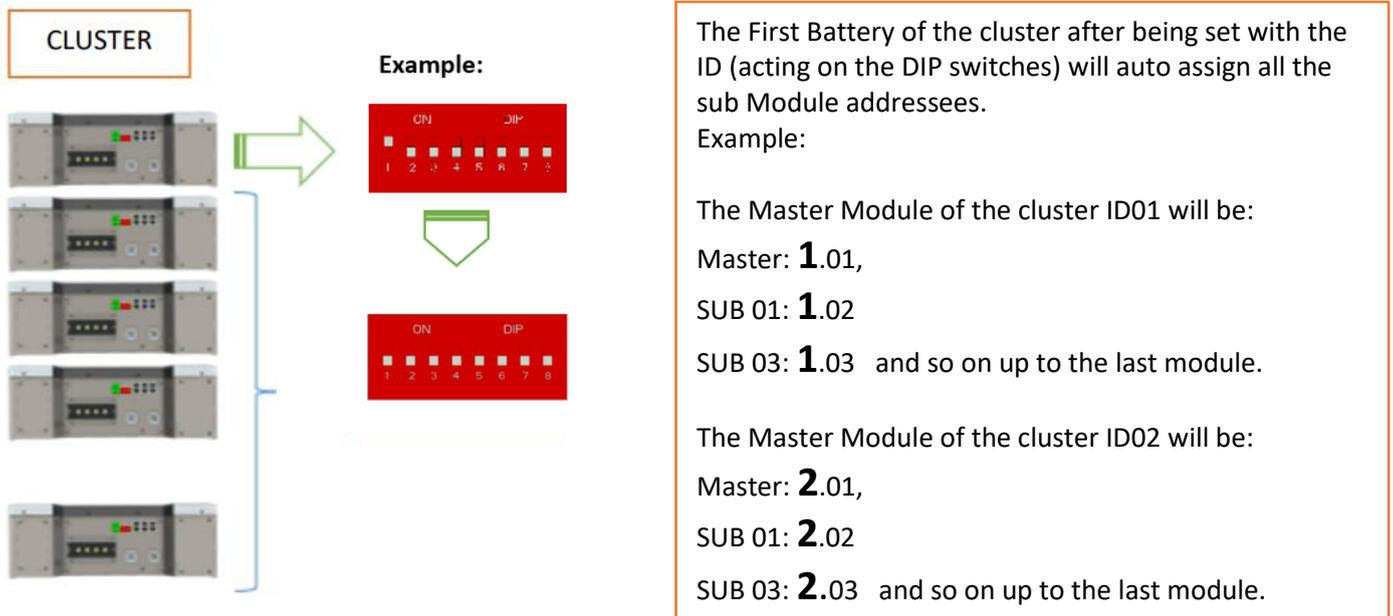
Only the first batteries of each cluster must be set following the sequence from ID 00 to ID 07 to allow the HUB to activate the related logic based on the number of modules present in each cluster (minimum 3, maximum 15), and based on the number of actual clusters connected to each other in a Daisy Chain (minimum 2 maximum 7).
