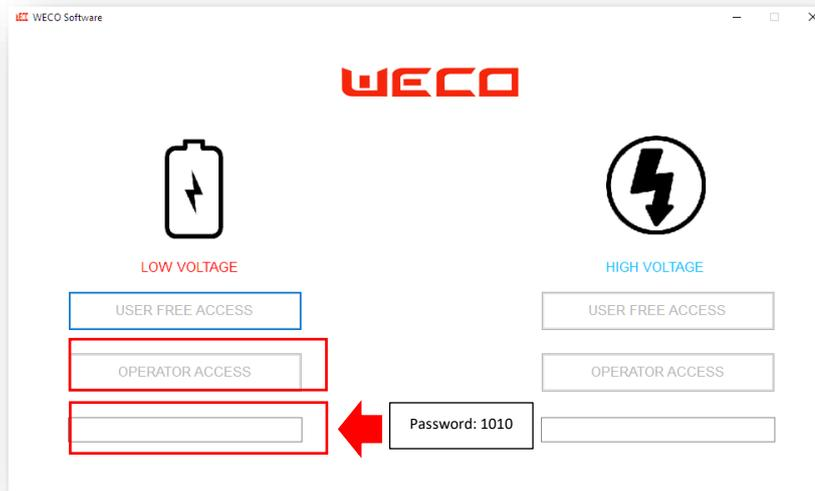
**STEP 2** Select the Single Module Setting Program after pressing OPERATOR ACCESS Button.
