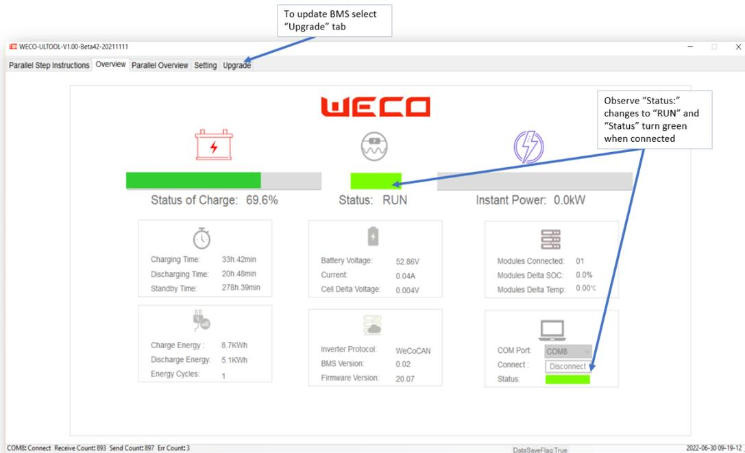
If more than one battery is connected in parallel, all the information will be displayed on this page. These pages will automatically update for up to 15 modules.
