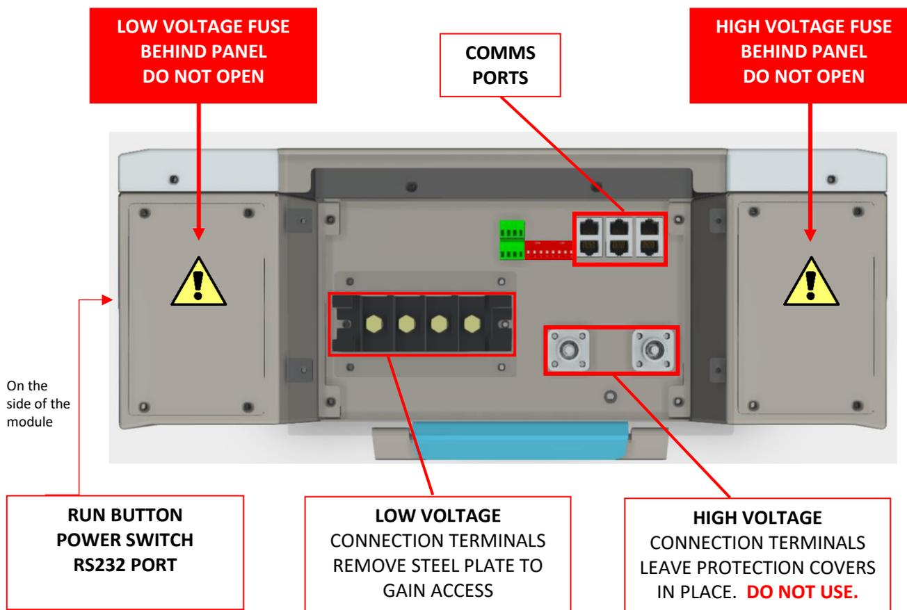
Note: The Run Button, Power Switch and RS232 Port are located on the right side when facing the unit. Deka label on the top.
