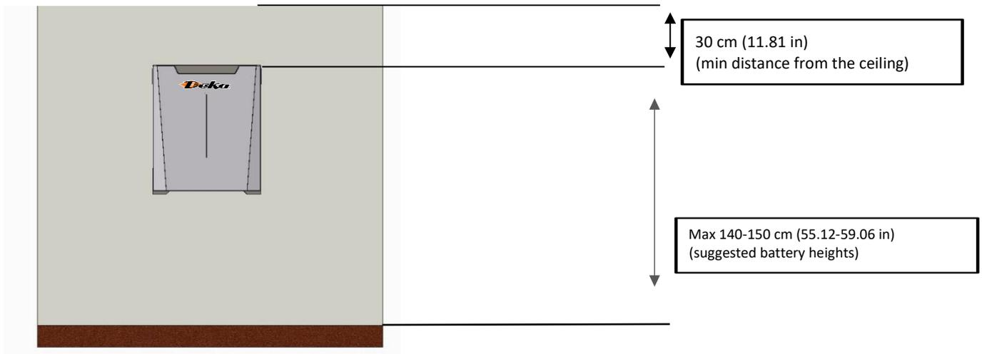
Step 2A: In case of multiple module installation, make sure to respect the distance between the modules and the ceiling.
