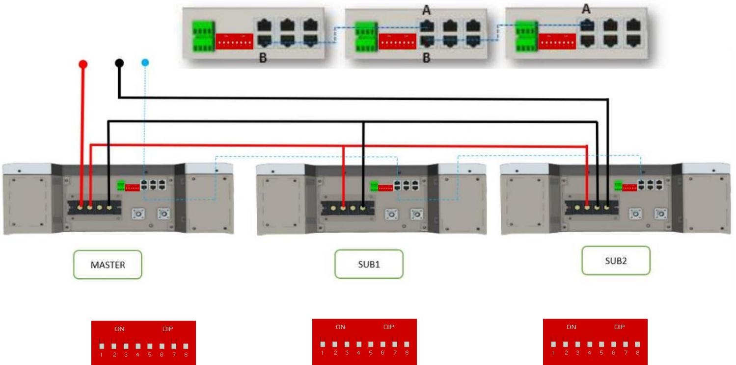
*Note: In a single cluster configuration, there is no need to set the DIP switch on the master battery. All DIP switches should be set to OFF. The single cluster will self-configure.*
