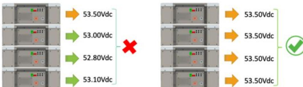
**It's recommended to individually charge all modules at the same level before proceeding with the final installation**
